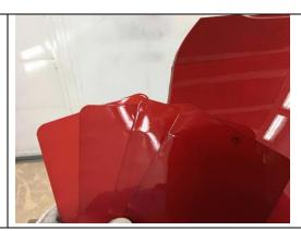
Check spray-out panels close to the repair and determine the amount of Mid-coat layers needed for imitating the OEM color.
