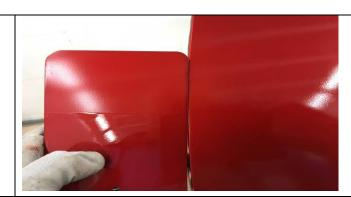
Check repair inbetween Mid-coats if the amount of coats applied is sufficient.
