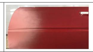
Apply Ground-coat according TDS respecting flash off times inbetween layers
