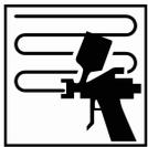
Apply one flowing coat of Autobase Plus toner Q070 to the entire area under repair.
