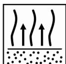
Allow each coat to flash-off naturally until the surface is completely matt.
