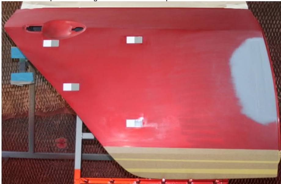
Picture 1 – Prepared and degreased area under repair
