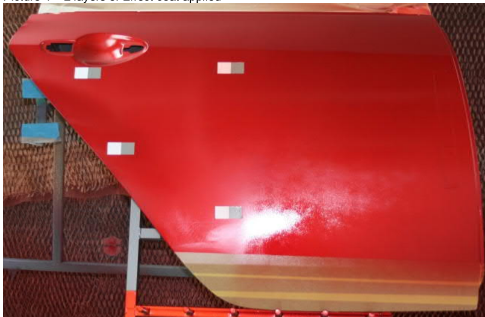
Picture 4 – 2 layers of Effect coat applied
